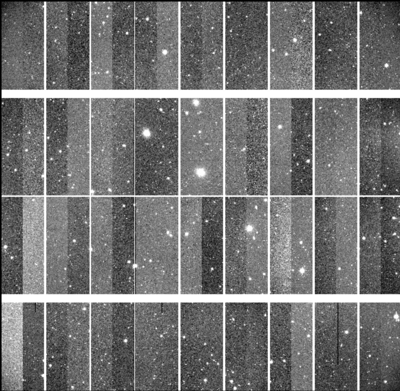
36 (2kx4k) CCDs, 2 readouts/CCD, 2x2 binning, unbinned (0.08"/pixel) ~800MB.
