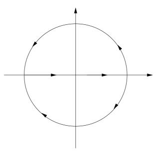
The integral along a contour containing a pole is a priory not well-defined. Such an integral must be treated as the limit of a well-defined contour integral, where the pole is "shifted" away from the contour by an infinitesimal amount. The manner, in which the pole is shifted, is usually imposed by the physical boundary conditions.
