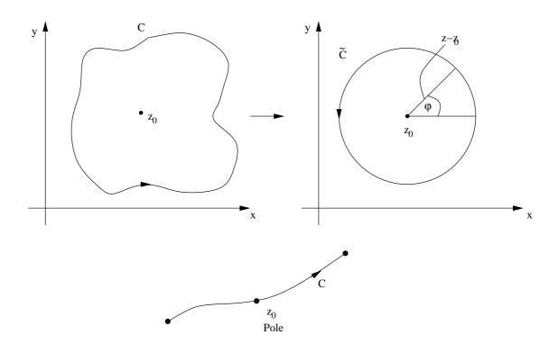
According to 4., the contour C can be deformed to a *circle*  $\widetilde{C}$ , without changing the  $\oint dz f(z)$ , such that  $z \in \widetilde{C}$  differs from  $z_0$  only by an infinitesimal number  $\varepsilon$ .
